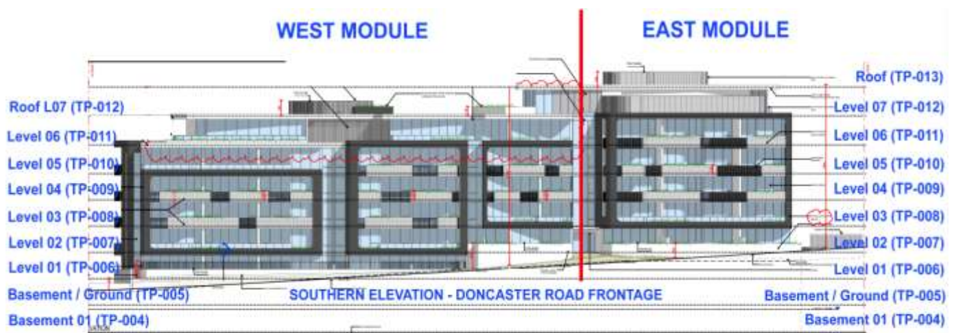
Figure 6: Southern Elevation with Plan Levels and Plan Page Number (reference Decision Plans)
