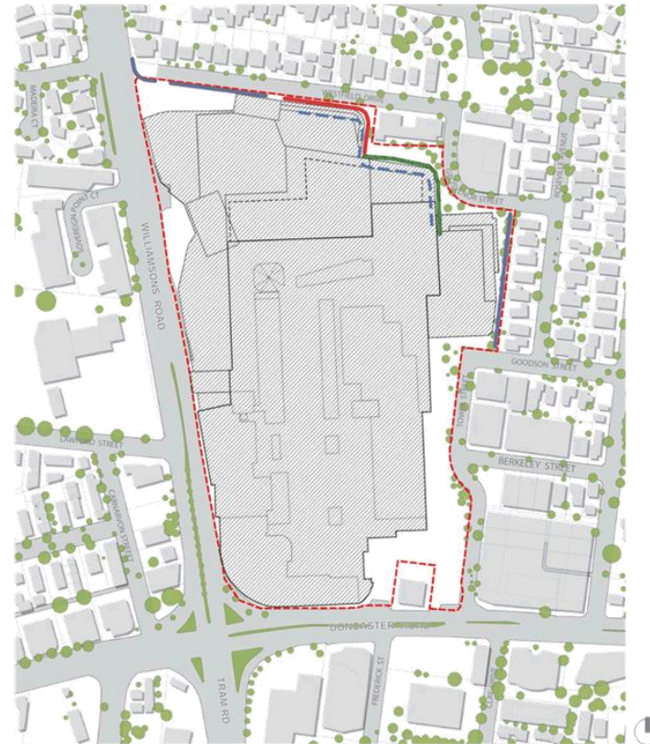
Figure 105: Proposed location of boundary acoustic treatments Key - - - Site boundary - Acoustic wall on boundary - 4.5m acoustic screen to Northern Boundary - 1.8m acoustic screen along ring road (upper level) - 1.2m acoustic screen along B4 carpark access (lower level) - Extent of acoustic screens as enclosure of carpark (level B5-Low@2)
