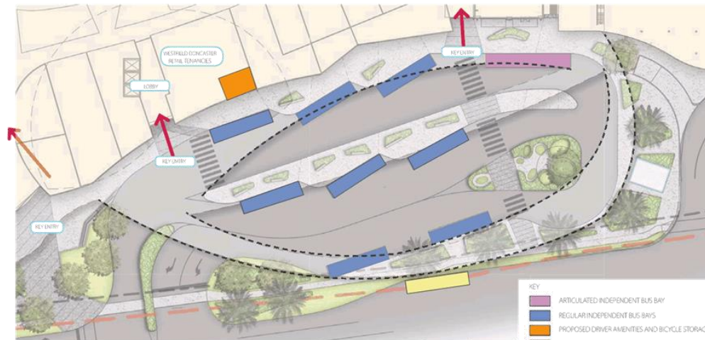
Figure 95: Proposed bus interchange concept plan showing configuration of nine bus bays and traffic layout
