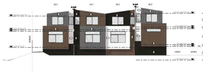
2 Townhouse - South Internal Elevation (D09-D12) 1:100
