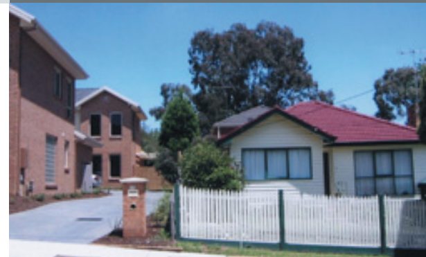
Lack of articulation and ground floor roof form adjacent to single storey development will emphasise height and visual bulk.
