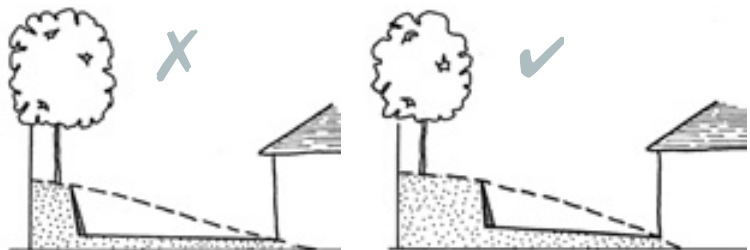
Excavating too close to an existing tree will impact on its health and longevity.
