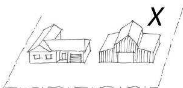
Figure 7- Inappropriate bulk and height of the outbuilding
