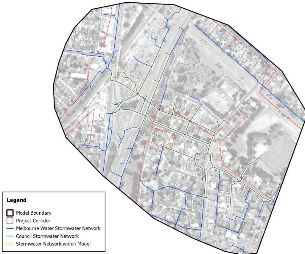
Figure 8-3 Watsonia Station Drain Model – Stormwater Network
